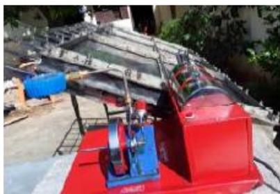
**Fig. 5. (a) Device with about 30 SPV cells with a packing factor of about 100% and about 2 litres  $\gamma$ -butyrolactone NWF and (b) the device connected to RMSE but not to the electric generator.**
