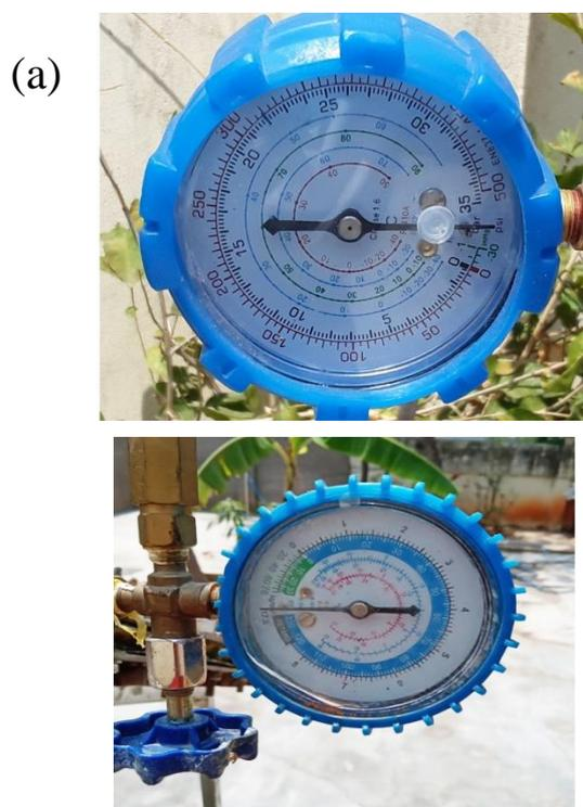
**Fig. 6. Pressure readings in two-different pressure gauges with two different scales with up to 35 bar and up to 8 bar connected to the manifold of copper conduit tube containing about 1.8 litre dichloromethane WF of the device that was exposed to the sunlight between 9 am to 1 pm on 29<sup>th</sup> March 2022 (a) and on 28<sup>th</sup> March 2022 (b).**
