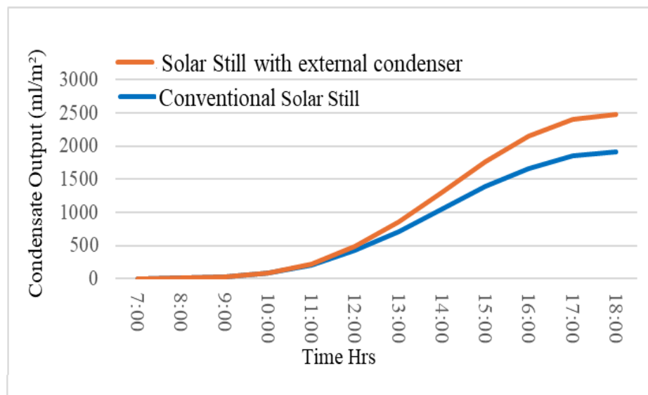
Figure 6b: Daily performance: conventional vs. condenser-enhanced solar still
