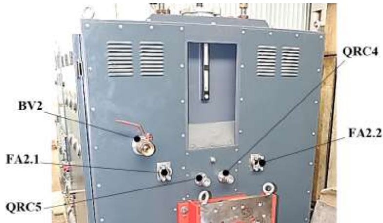
Figure 5. Elements of the right side panel of the test bench: FA2.1, FA2.2 – flange adapters of high-pressure lines; BV2 – auxiliary supply valve; QRC4, QRC5 – quick-release couplings of the hydraulic motor drain circuit.
