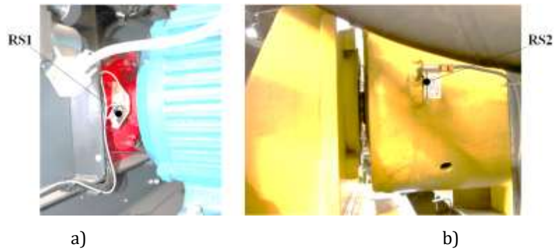
Figure 7: Hydraulic machine shaft rotation sensor assemblies: a – pump; b – hydraulic motor
