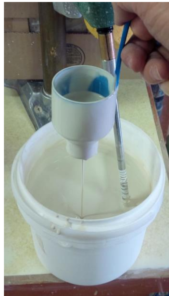
Figure 2. In the art room, a Ford cup is used to adjust and measure the viscosity of liquid slurry poured into a mold by calculating the time that the liquid passes through a hole in the bottom of the cup
