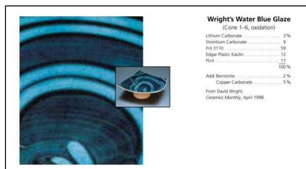
Figure 1. Glaze recipe including all four groups of ceramic glazing materials (glass formers, fluxes, refractories, and colorants) (source: Sierra Nevada College, www.ceramicartsdaily.org , 2013)
