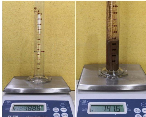
Figure 4. Measuring the specific gravity of an ACTP clay slip (SQU Ceramics Lab) (source: Badar Almamari, JSBAR, 2020)
