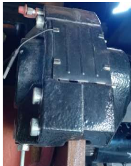
Figure 2: (A) Right brake caliper; (B) Left brake caliper
